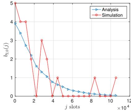
Fig. 12. Number of RACH successes in a radio frame for 3GPP EAB mechanism in Case 2
