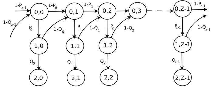
Fig. 6. State diagram of proposed fast RACH mechanism
