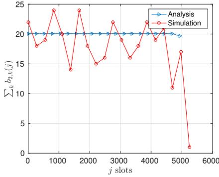
Fig. 10. Number of RACH successes in a radio frame for FRM in Case 1
