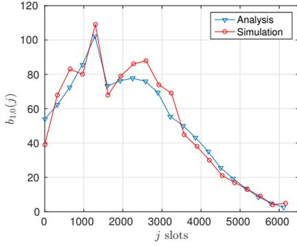
Fig. 7. Number of RACH attempts made in a radio frame for 3GPP EAB mechanism in Case 1
