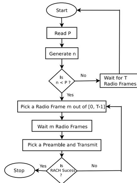
Fig. 2. 3GPP extended access barring mechanism
