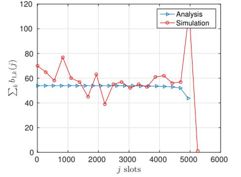
Fig. 9. Number of RACH attempts made in a radio frame for FRM in Case 1
