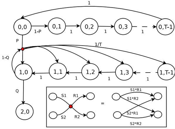
Fig. 5. State diagram of existing 3GPP extended access barring mechanism
