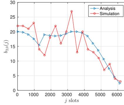
Fig. 8. Number of RACH successes in a given radio frame for 3GPP EAB mechanism in Case 1
