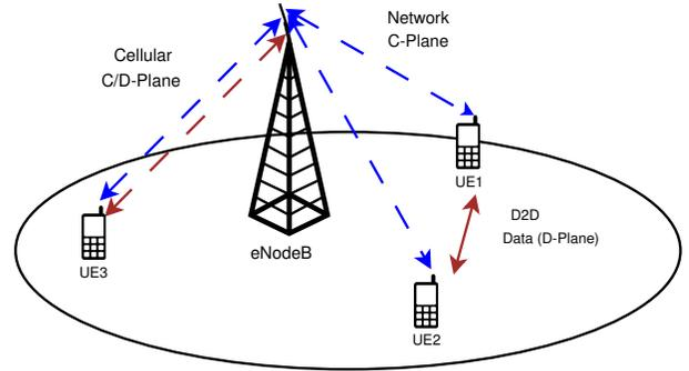
Fig. 1. Typical example of traditional cellular and D2D communication
