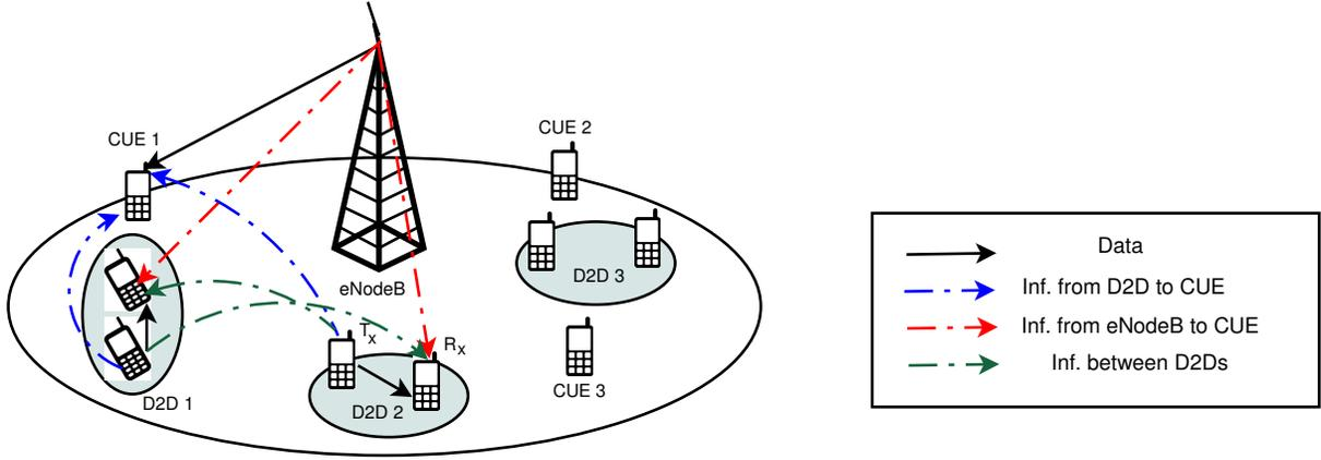
Fig. 2. D2D System Architecture
